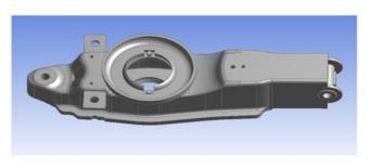
Fig. 3.1 Model of Wishbone Arm
