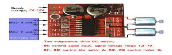
Fig 3: L293D Motor Driver
