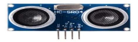
Fig 5: Ultrasonic sensor
