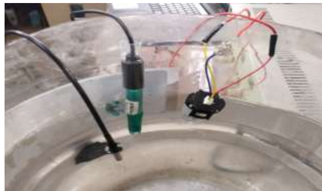
Fig-4: Sensor Installation in Water Tank
