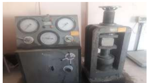
Fig:-4 COMPRESSIVE STRENGTH TEST
