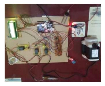
**Fig -11**: Final working model of smart irrigation with incubation system using Arduino Uno
