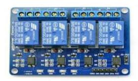
Fig -4: 4-Channel Relay Module
