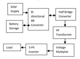
Figure 1: Grid connected system with voltage multiplier for three phase applications.
