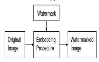
Figure 1: Embedding process of image watermarking [1]
