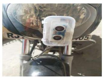
**Fig-1**. Ultrasonic Emitter and Receiver Mounted on Motor Bike
