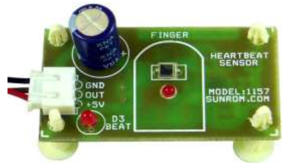
Fig-3: Heart Rate Sensor Sunrom 1157
