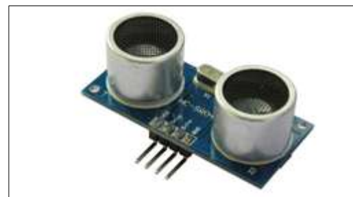
Fig 3. HC-SR04 Ultra-sonic Sensor
