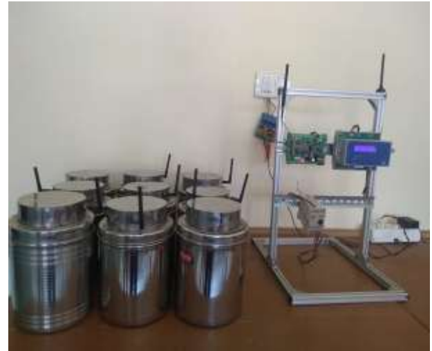
Fig 14. Full model of smart container using Ultrasonic sensor
