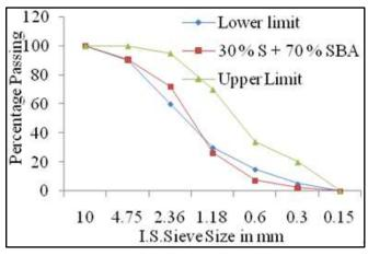
Fig -4: Grain Size distribution curve
