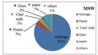
Fig -2: Characterization of solid waste
