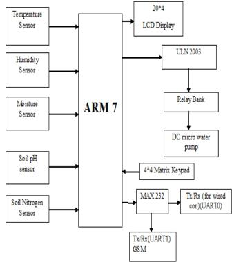
Fig -1: System Block Diagram
