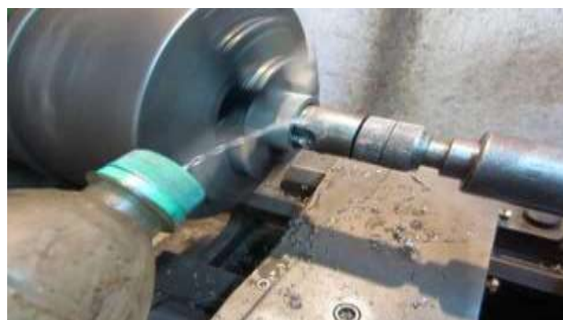
Fig. 5. Hex Key Cutting Operation
