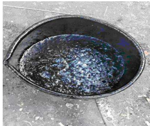
Figure 2 sample of foamed bitumen
