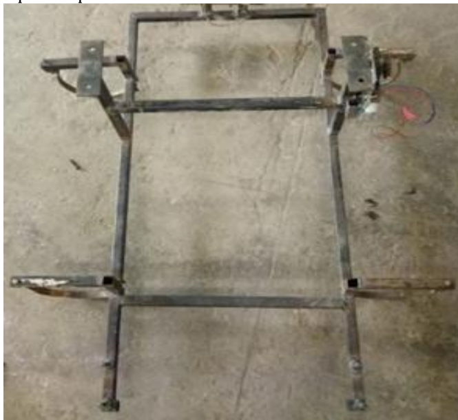
Fig-7.1: Base Frame of River Cleaning Machine
