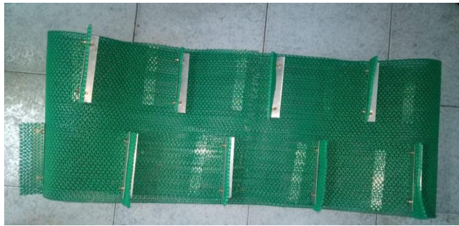
Fig-7.10: Conveyor Belt
