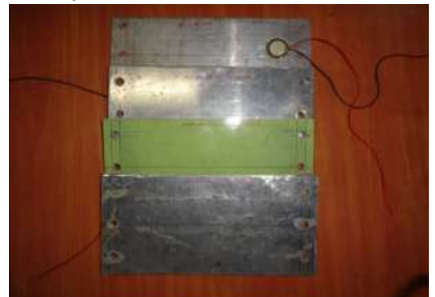
Figure 3.2: AL Plates with piezo patch
