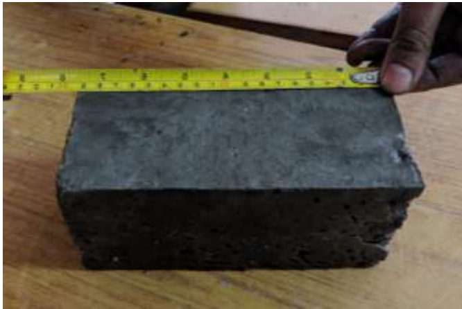
Fig -1: C&D Waste Brick
