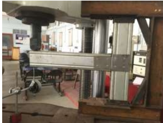
Fig 2-1: Experimental Setup of Model with loading frame.
