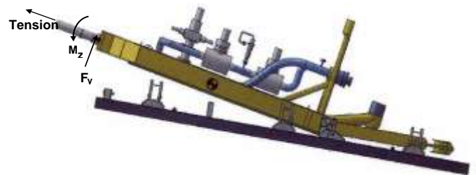
Fig 8:-Installation Loads on Typical FTA
