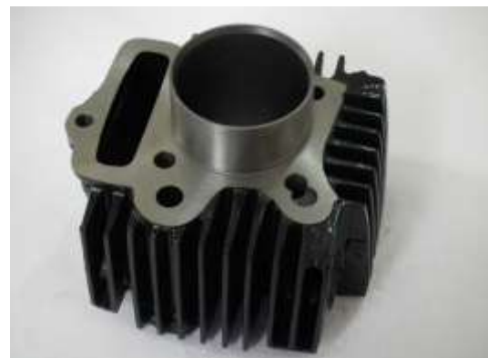
Figure 1.1: Photographic View of Existing Cylinder Block with fins
