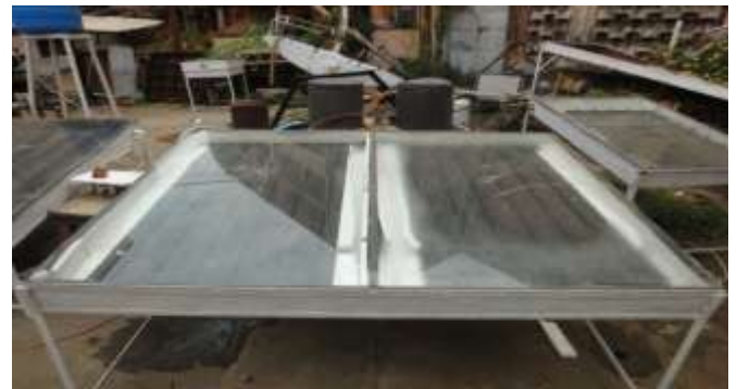
Fig-1: combined flat plate liquid solar collector
