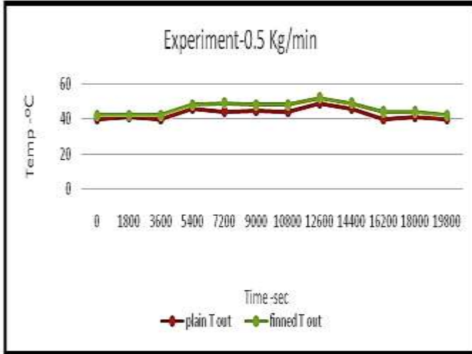
Graph-2: temp vs time at 0.5kg/min (exp)
