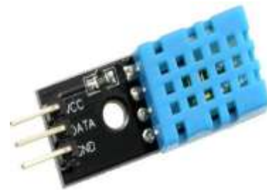
Figure 5. Air temp & humidity sensor
