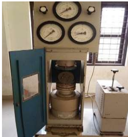
Fig-3: Cylinder testing in compression testing machine
