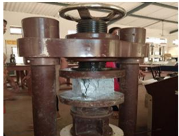
Fig1 : compressive strength test
