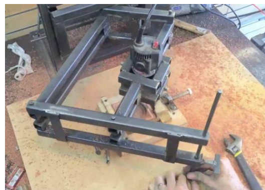
Fig 2: Model of Portable Pantograph
