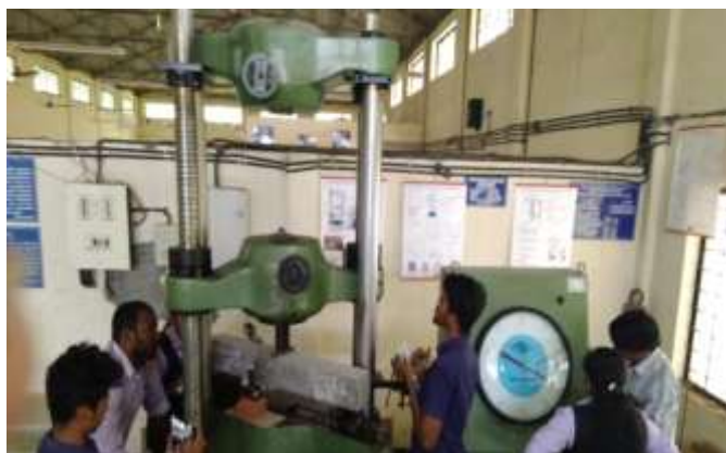
Fig -16: Testing of strengthened beam in UTM
