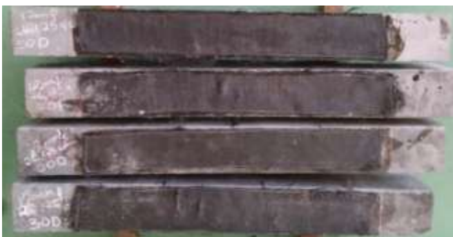
Fig -15: Installation of CFRP sheets after making holes
