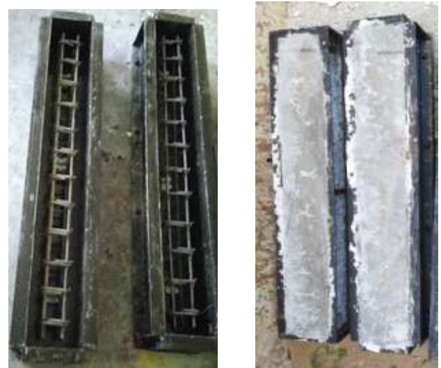
Fig -11: Stages of beam casting
