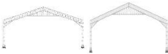
Fig -3: CSB (span 50m , 60m)
