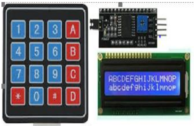
Fig. 6. 4*4 Matrix keypad and 16*2 LCD with I2C
