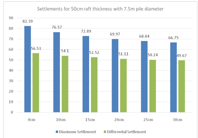
Figure 28:- Displacements of piled-raft with 50cm raft thickness and piles of length 7.5m at different diameter.
