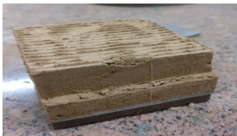
Figure 3:- Shear failure of soil samples
