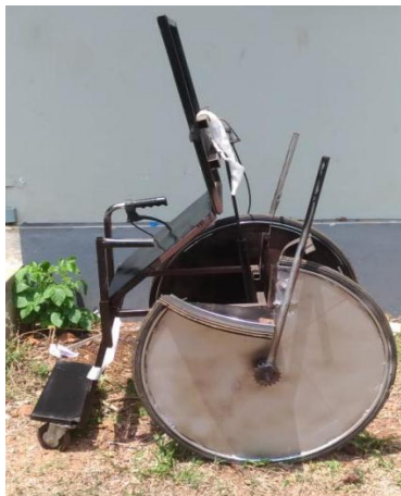
Fig 10.2 Mechanical Assisted Wheelchair in Standing Position
