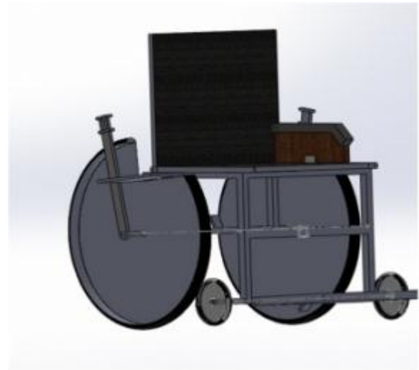
Fig 5.1: 3D CAD model of Wheelchair Design
