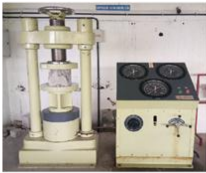
Fig.3: Compression testing machine
