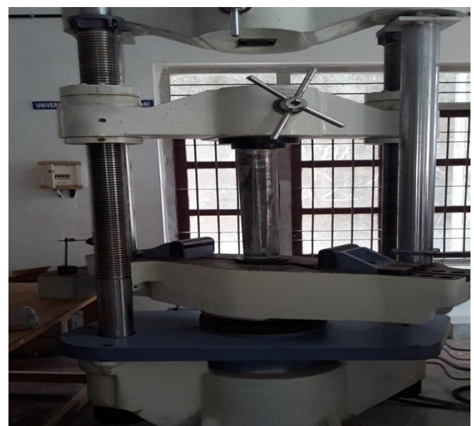
Fig-2: Test setup of column specimen
