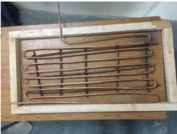
Fig -1: Wooden Frame, Reinforcement, Copper Pipes
