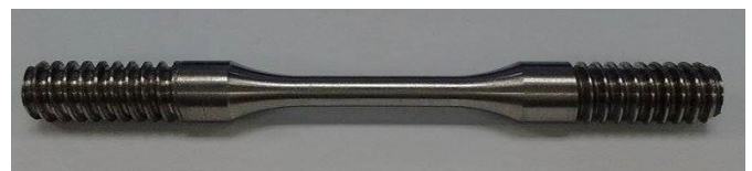
Fig -3.3: Typical specimen after machining
