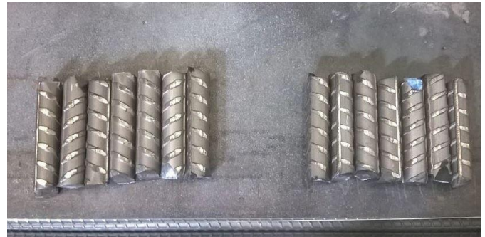
Fig -3.1: Rebar cut pieces before machining to desired shape
