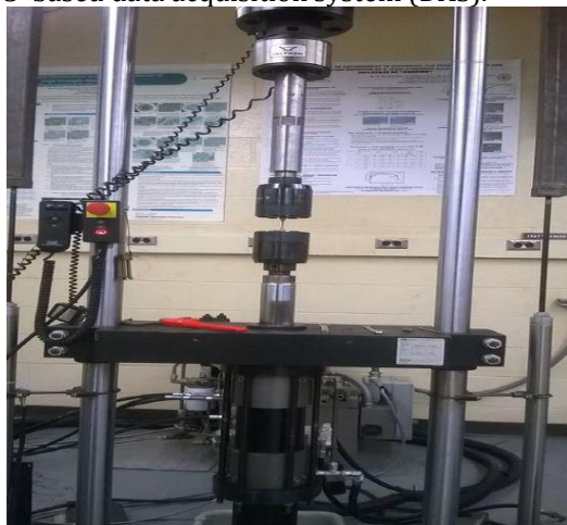
Fig -4.2: Test setup for tensile testing at room temperature
