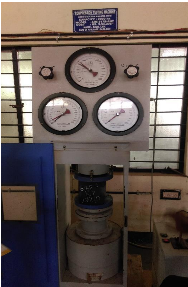
Fig.1 Compressive strength test set up
