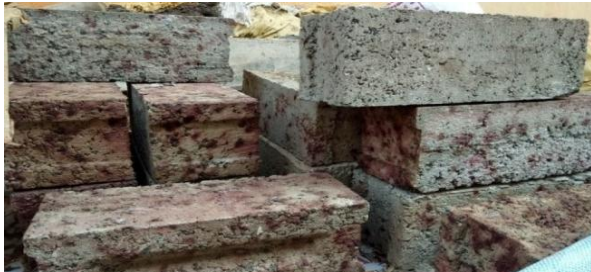
Fig - 5: Cast Solid block for various proportions of waste bakelite
