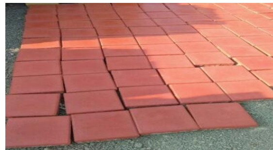
Fig - 6: Cast Paver block for various proportions of waste bakelite
