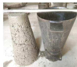
Fig -2: Slump test
