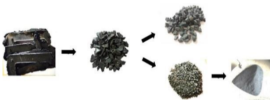
Fig -1: Processing & Classification of waste bakelite
