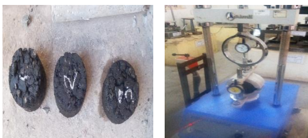
Fig -4 & 5: Specimen after 24 hours curing period & Marshall testing Apparatus
