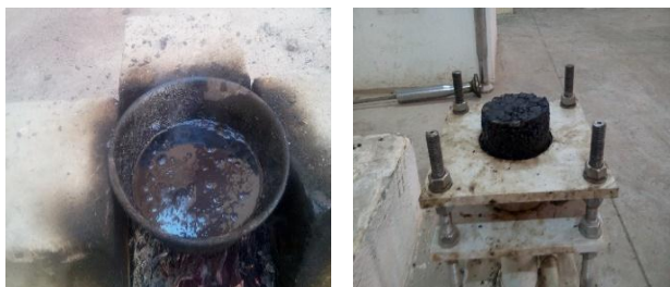
Fig -2 & 3: Preparation of hot bitumen & Extraction of bituminous specimen from the mould
