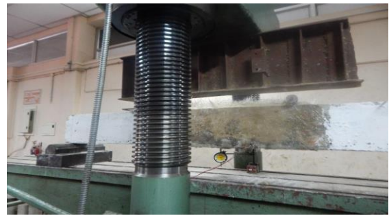
Fig -3: Testing of U wrapped specimen (U3)
