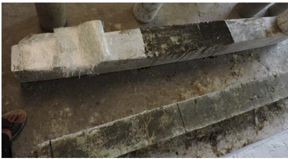
Fig -2: Application of Epoxy Resin layer on specimen
