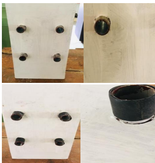
Fig -1: Mild Steel pipe connectors (i) Without rubber sleeve ( S ) (ii) With rubber sleeve (RS)
