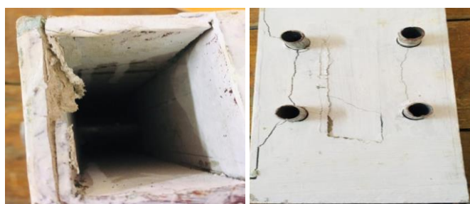
Fig -6: Failure mode of steel specimen (S2)
