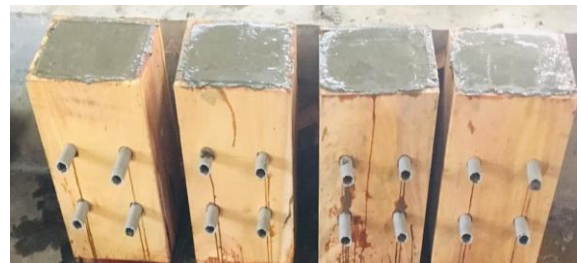
Fig -2: Timber blocks cast with pipe connectors
