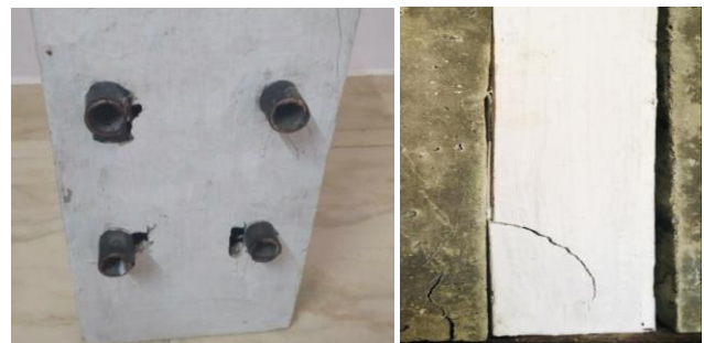
Fig -7: Failure mode of Rubber Steel pipe Specimen (RS1)
