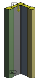
Fig -1: Boundary conditions and lateral loading
