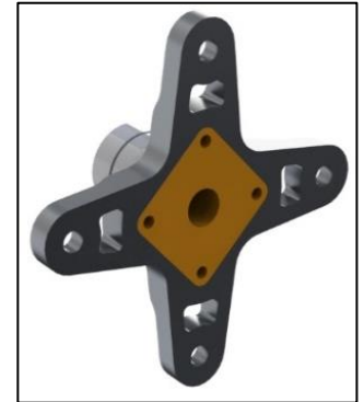
Fig.2.b New Hub Design With Insert
