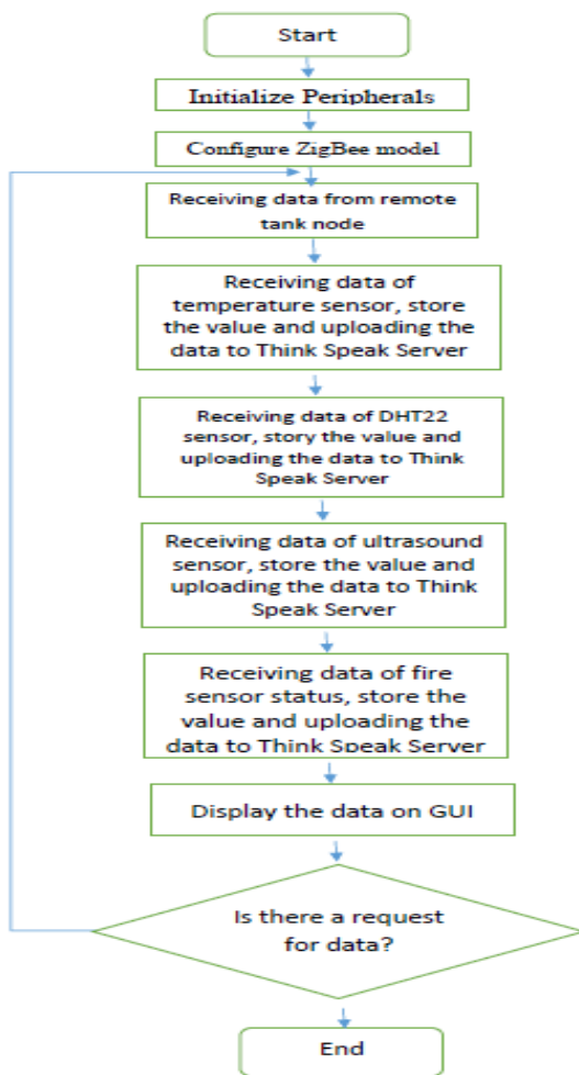
Fig -5: Flowchart of Coordinator node
