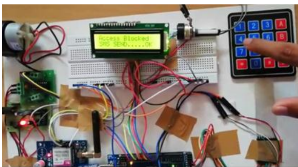
Fig 6 SMS is send to the authorized person when password entered is wrong
