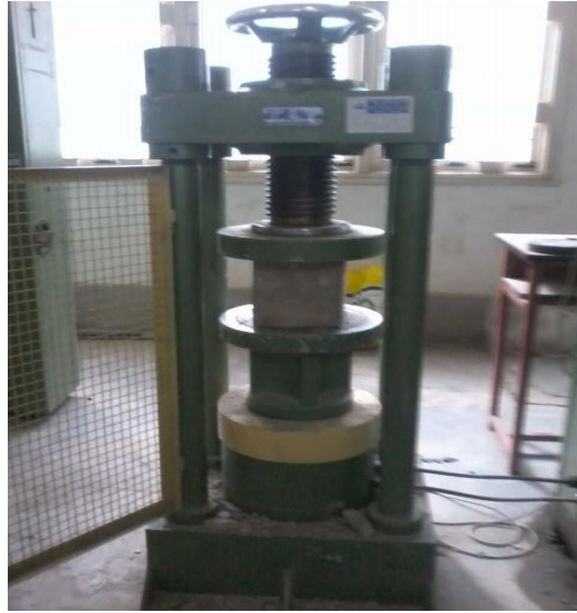
Figure 2 Compression test setup
