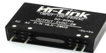
Fig6.4. SMPS power supply (230v AC-5VDC)
