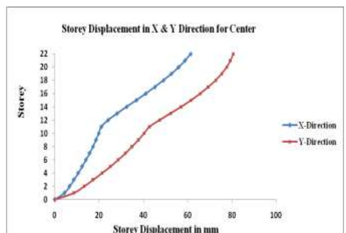
Figure 5: Storey displacement for irregular position for center along X and Y direction
