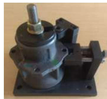
Figure -8: Fixture with NRV Body component
