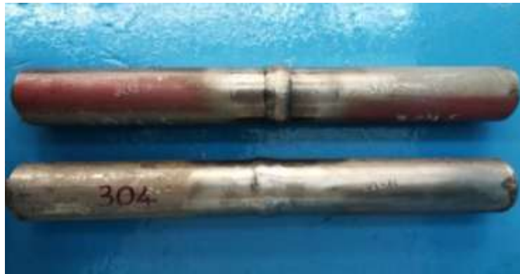
Fig 1.5 Welded samples of similar joint of super 304H tube
