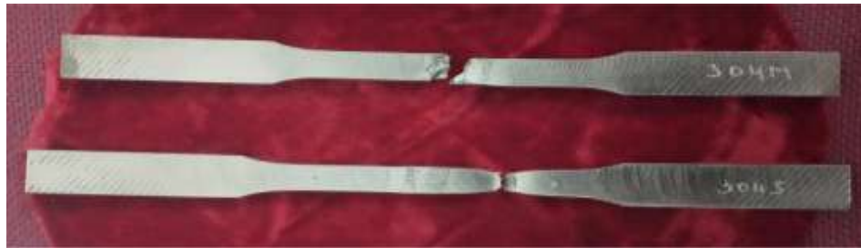
Fig 2.1 Tensile test of manual and semiautomatic welded sample
