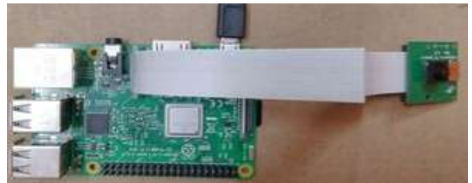
Fig -5: Interfacing Camera Module with Raspberry Pi
